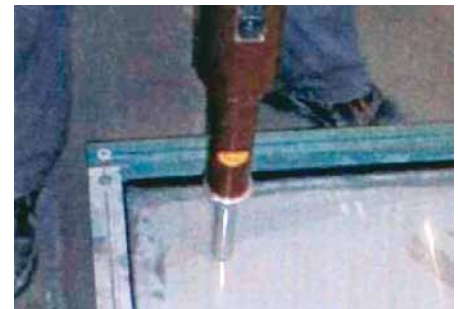
POINT 1 - EDGE IMPACT WITH CONCRETE TESTING HAMMER
